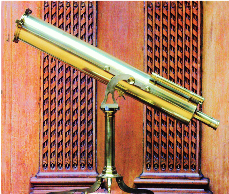
Gregorian reflecting telescope, P and J Dollond, London, pre 1789
